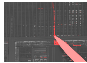
EBAC on a semiconductor sample
